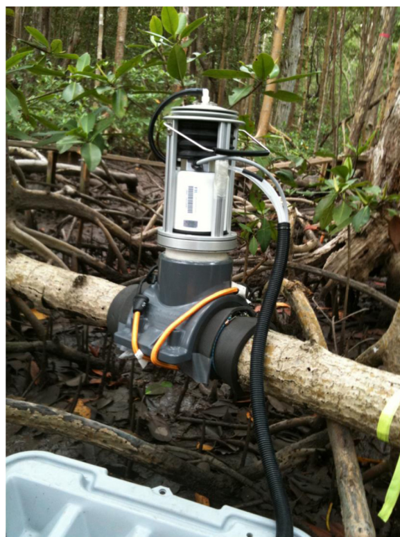
Fig. 2. Measurement technique for \text{CO}_2 flux from coarse woody debris. LI-COR 8 cm chamber affixed to a downed tree using a PVC saddle T, silicone foam and elastic cords.
